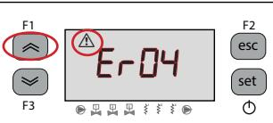
Repair the fault before performing the reset.
