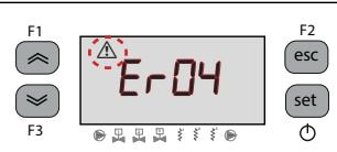
press the button "esc" until the alarm disappears.
